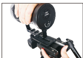
19 Press the red button on tripod to fix the plate onto tripod.
