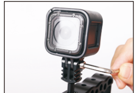
13 Screw the GoPro onto the connector with the bolt.
